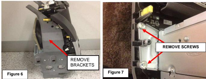
**9.** Remove the 2 x screws from either side of the audio module holding it in place and remove the cable tie attached to the top of the chassis holding the cable in place.
