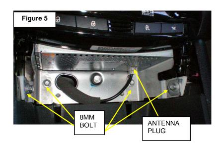
**8.** Remove 4 screws holding the TFT screen to the facia.
